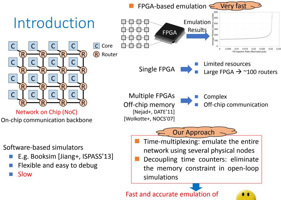
large NoC designs on a single FPGA
